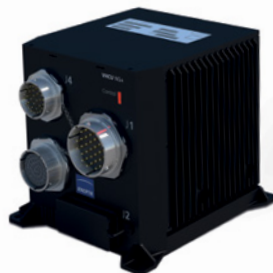
VHCU NG+ (8/12 channels, design model)
